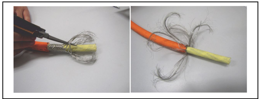
Fig. 5-5: Split the shield braid open
