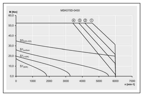
Fig.4-45: Characteristic curves MSK070D-0450
