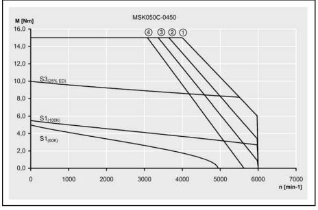
Fig.4-24: Characteristic curves MSK050C-0450
