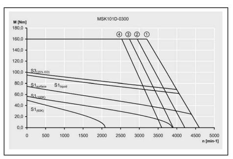
Fig.4-100: Characteristic curve MSK101D-300
