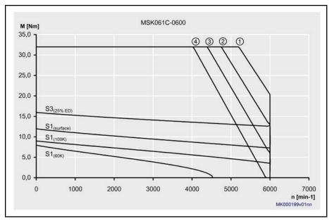
Fig.4-37: Characteristic curves MSK061C-0600
