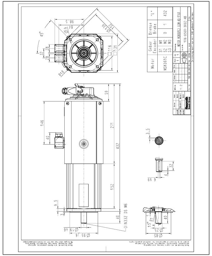
Fig.5-11: MSK061 specifications with axial fan unit
