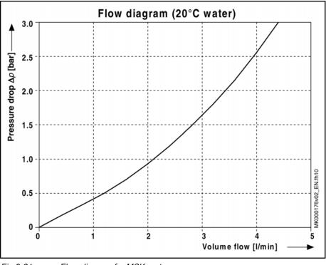
Fig.9-21: Flow diagram for MSK motors
