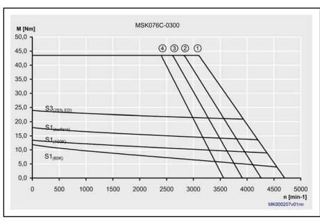
Fig.4-75: Characteristic curves MSK076C-0300
