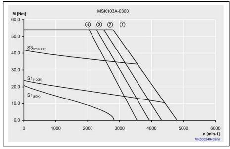
Fig.4-107: Characteristic curve MSK103A-0300
