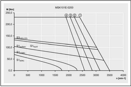
Fig.4-103: Characteristic curve MSK101E-0200
