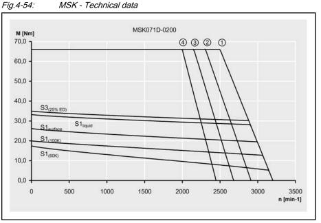
Fig.4-55: Characteristic curves MSK071D-0200
