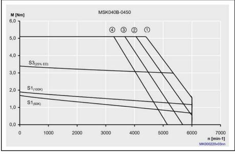
*Fig.4-11: Characteristic curves MSK040B-0450*
