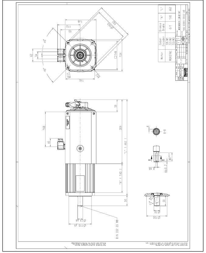
Fig.5-25: MSK076 specifications with axial fan unit
