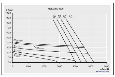
Fig.4-72: Characteristic curve MSK075E-300
