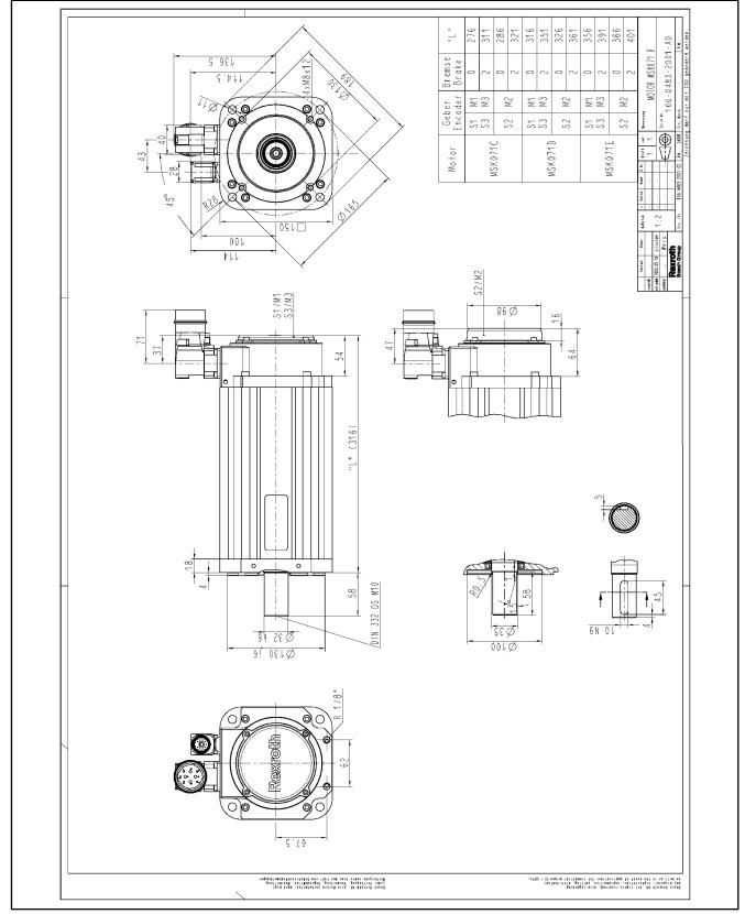
Fig.5-17: MSK071...FN specifications
