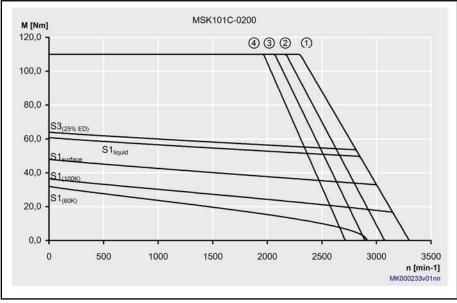
Fig.4-95: Characteristic curve MSK101C-0200
