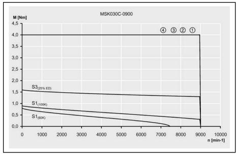
Fig.4-9: Characteristic curves MSK030C-0900
