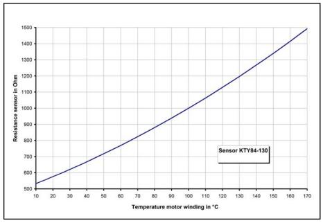
Fig.9-24: Characteristic curve KTY84-130
