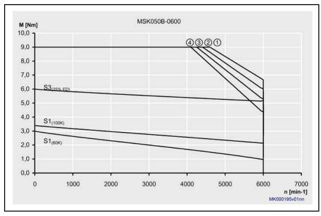
Fig.4-21: Characteristic curves MSK050B-0600
