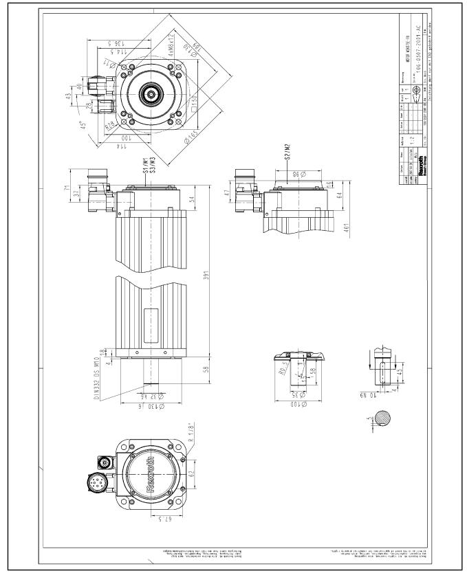
Fig.5-21: MSK075...FN specifications
