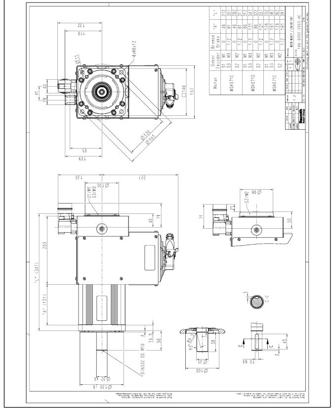
Fig.5-19: MSK071 specifications with radial fan unit
