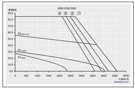
Fig.4-109: Characteristic curve MSK103B-0300
