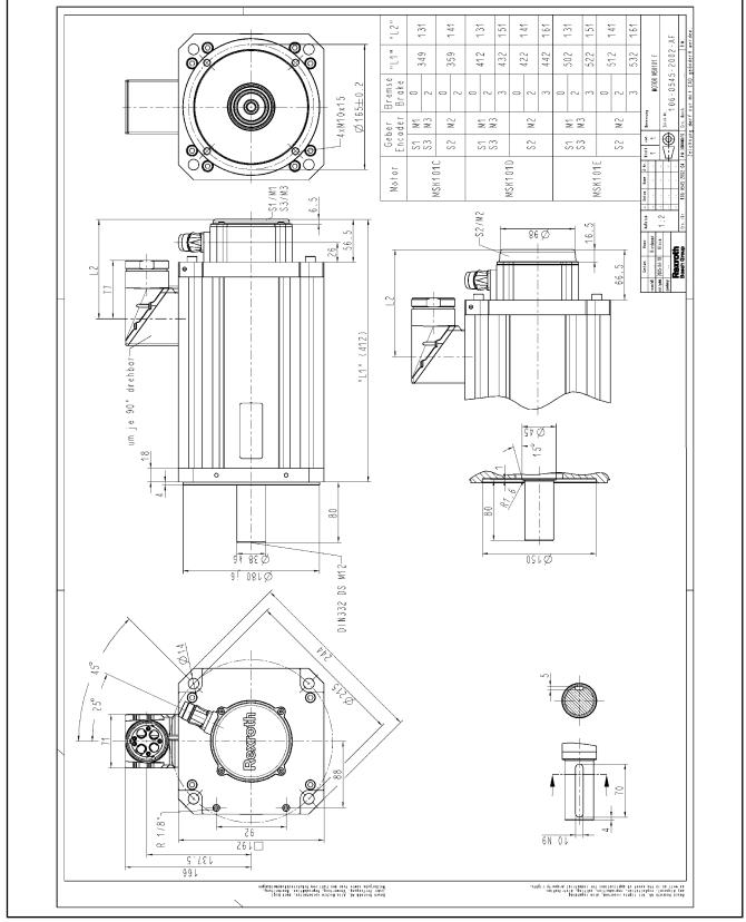
Fig.5-31: MSK101...FN specifications
