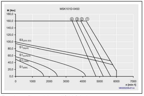
Fig.4-101: Characteristic curve MSK101D-0450
