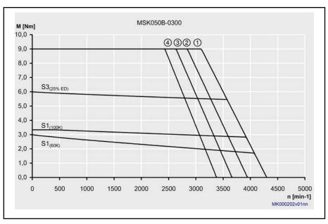
Fig.4-19: Characteristic curves MSK050B-0300
