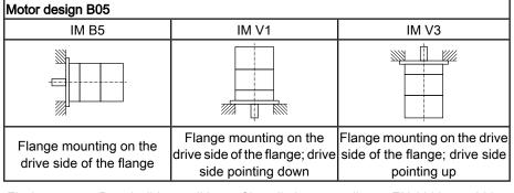
Fig.9-7: Permissible conditions of installation according to EN 60034-7:1993
