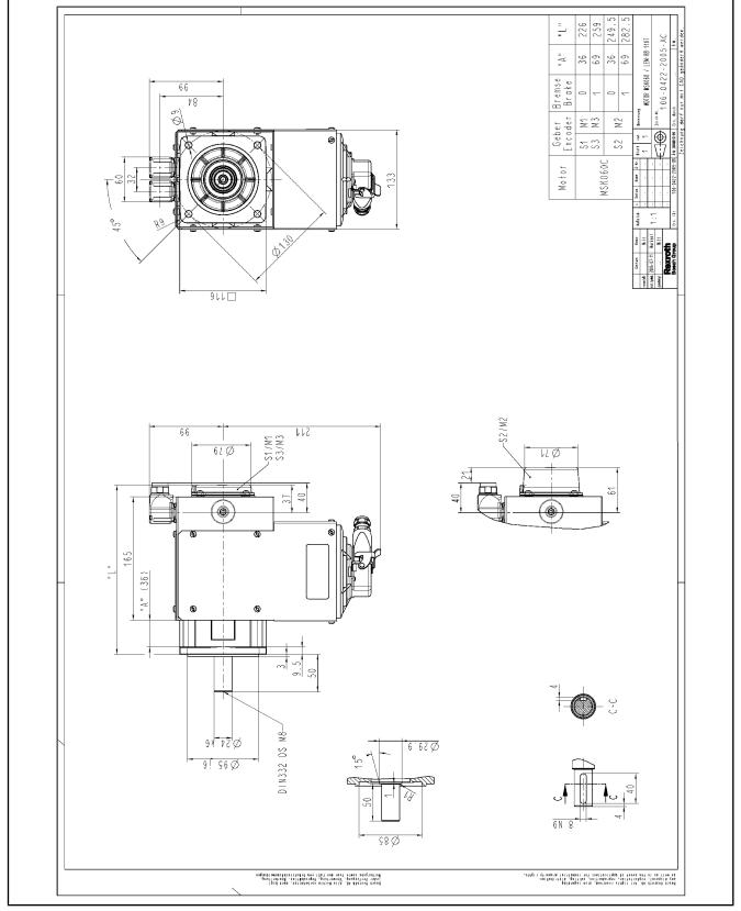
Fig.5-9: MSK060 specifications with radial fan unit
