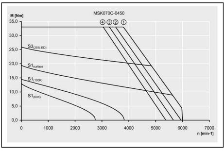
Fig.4-41: Characteristic curves MSK070C-0450
