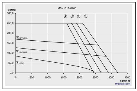
Fig.4-113: Characteristic curve MSK131B-0200
