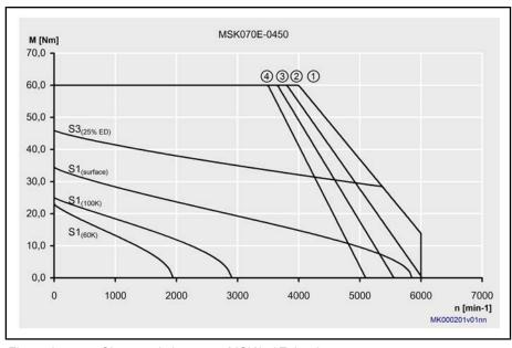
Fig.4-49: Characteristic curves MSK070E-0450
