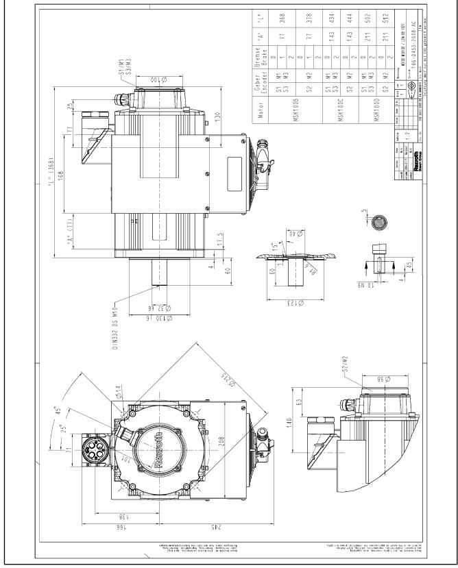
Fig.5-29: MSK100 specifications with radial fan unit
