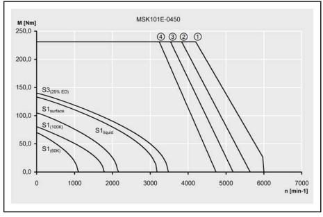
Fig.4-105: Characteristic curve MSK101E-0450
