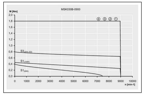
Fig.4-7: Characteristic curves MSK030B-0900
