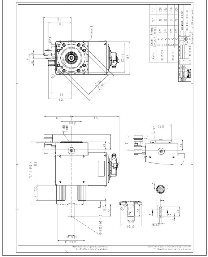
Fig.5-15: MSK070 specifications with radial fan unit
