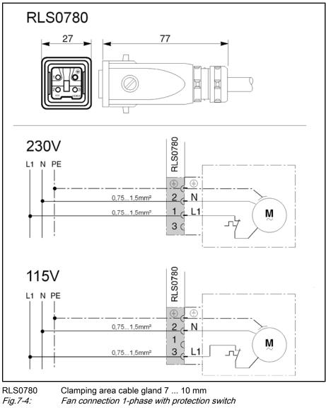
LEM fan units in design "T" with integrated thermo protection do not need any circuit with external motor protection switch.
