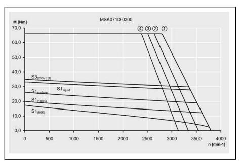
Fig.4-56: Characteristic curves MSK071D-0300
