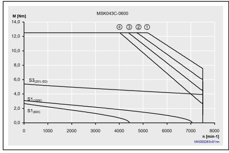
Fig.4-17: Characteristic curves MSK043C-0600
